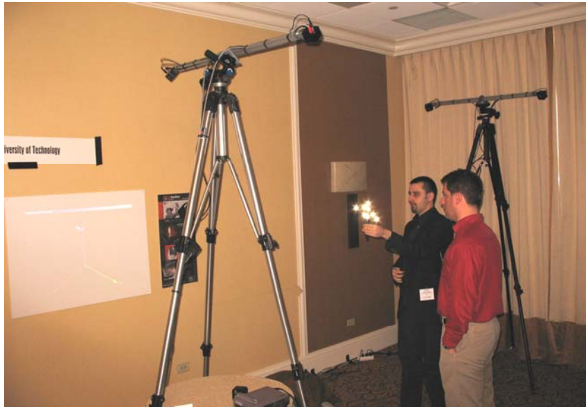
Figure 2: Infrared based optical tracking system iotracker from Vienna University of Technology.
