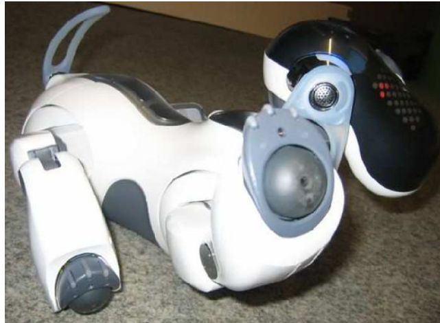
Figure 1: The AIBO used for the experiments during a learning phase. The robot can perform all physical possible movements in order to try to move forward, as long as they are symmetric and do not put too much force on the joints. The binary touch sensors on the paws are also fed into the neural network, together with the position of the joints and the intended movements of these joints.
