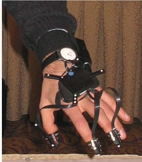
Figure 3: Tactile feedback device by VW Group Research and Bauhaus-University Weimar.
